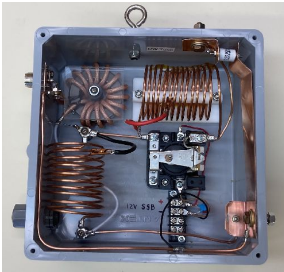
Fig 8. Complex 80m vertical feed point box with hairpin coil, CW-shift coil with a relay, choke, and lightning arrestors. This box is bolted to Unistrut.
