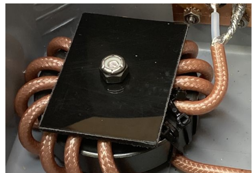
Fig 3. A toroidal choke clamped in place with a piece of 1/8 in. acetal and a machine bolt.
