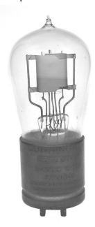
long pin UX bases. This was an improvement in the electrical contacts and made the tubes easier to use in production radio sets.
