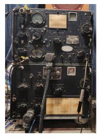
I decided I needed an iambic keyer for the TCS set. I remember reading that there is high voltage across the key contacts -- if I remember correctly it is more than 100 volts, so a normal 2N2222 single transistor keying circuit wouldn't work.
