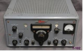
Both RX and TX bear a visual similarity to the Collins 75Sx/32Sx series, the architecture was the same, and both copied the permeability-tuned oscillator [PTO] and the ganged tuning rack from the S-line. Eldico also offered the speaker/power supply/control modules similar to the Collins 312B series. Cheaper than Collins and with lesser but acceptable quality, they found their way into many ham shacks in the 60's/70's.
