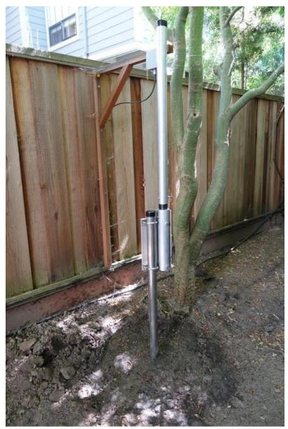
The compromise radials will be replaced with a zinc galvanized wire cloth as mentioned in Jim K9YC's excellent <u>Pacificon presentation</u>. I have and extremely limited space for this antenna, as you can see in the photograph, so maximizing the radial system in this way makes sense to me.
