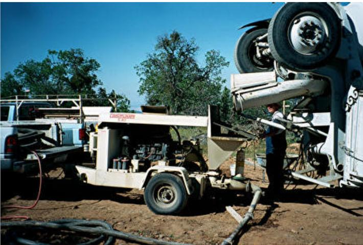
Concrete pumps are truly slick machines! Here is the business end. It pumps mud through a two inch hose.
