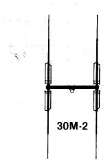
30M-2: SPECIFICATIONS Bandwidth: 10.1 to 10.150 MHz Gain:
