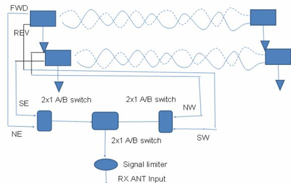
Each head-end box implements a bi-directional beverage. The box in the upper left-hand of the figure is NE/SW; the other
