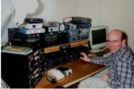
Here's Bob at the wheel of N6TV. The two boxes to his left are his keyer and the manual A/B rig switching control box.
