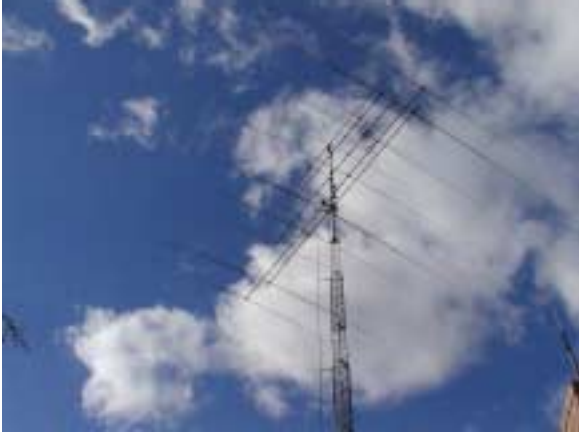
N6TV's antenna system sits on a single 89-foot tower. At the top is an 80 m rotary dipole. At the bottom is a 3-element 40 m yagi. In between, from bottom up, are 5 element monobanders for 20, 15 and 10.
