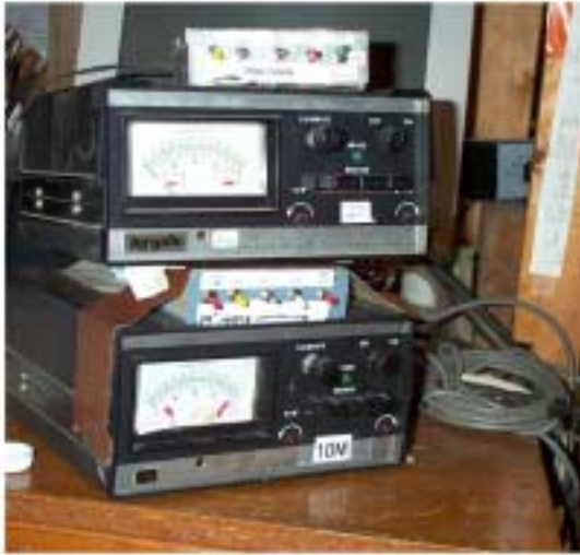
Rotator and stack-switching controls for the 10 and 20 meter stacks.
