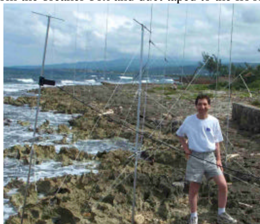
Kenny, K2KW, by the 2-element Sigma-6 array. Behind him are the 4 element 10M European array, 4 element 15M European array, 2 element 80M array, and 160M inverted L.
